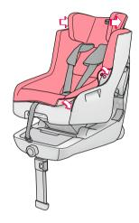
Attach the cover by way of the snap fasteners on the CONCORD ABSORBER.
