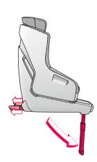
Set down the CONCORD ABSORBER in drive direction onto the seat or the seat bench.
