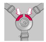
To open the harness system, press the button in the middle of the buckle until the buckle adaptors are released.
