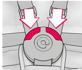
To open the harness system, press the button in the middle of the buckle until the buckle adaptors are released..
