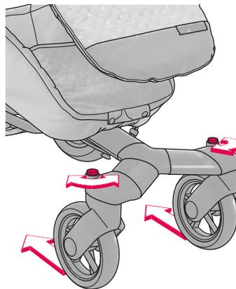
Position the front wheels of the CONCORD NEO to face backwards, and turn the locker buttons (09) from the outside inwards to lock the front wheels.
