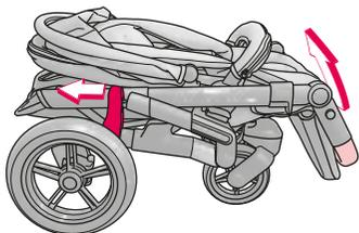
To fold down the CONCORD NEO, first adjust the seat angle on the seat frame (03) to position P (see ADJUSTING THE SEAT ANGLE).
