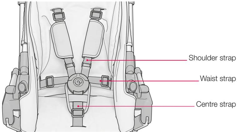
Feed the centre strap with the buckle between the child's legs. Then insert the buckle adaptors on the shoulder and waist straps from above into the top of the buckle. They should click audibly into position.
